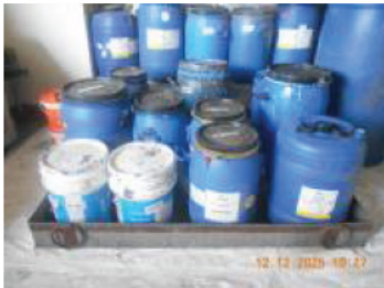
Secondary containment provided to ink containers.jpg
