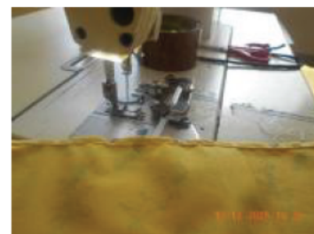
Needle guard provided to the stitching machine.jpg
